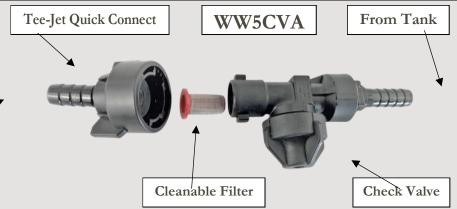
This assembly comes pre-installed to the inlet side of the manifold. Make sure that you have a way to turn the pump on and off. You will not be running the pump continuously while using your weed wiper. When the pump is on, chemical will be pumped into the PVC, then through small holes saturating the sponges. This pump fed system will ensure quick filling and instant shut off since the system in pressurized.
