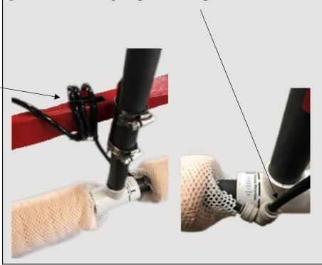
Step #11 Check Valve & Filter Assembly
