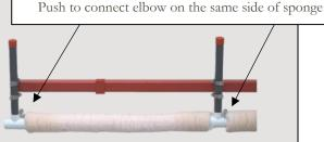
Notice the trisers are attached in the same spot to ensure a level sponge boom. Additionally, make sure that you clamp each t-riser at the same height to ensure that your sponge boom is level. After finishing these steps, make sure you stretch your sponge out over the t-risers so that your boom is almost entirely covered by your sponges.
