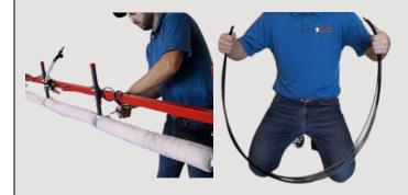
Simply push the tubing into the quick connectors on both your sponge section, and your manifold (as shown above). Any extra tubing can be coiled up and zip tied down to the boom. Do not over tighten the zip ties and pinch the tubing. The manifold pictured below is a 4-port manifold, you have two 6-port manifolds.
