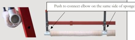
Notice the trisers are attached in the same spot to ensure a level sponge boom. Additionally, make sure that you clamp each t-riser at the same height to ensure that your sponge boom is level. After finishing these steps, make sure you stretch your sponge out over the t-risers so that your boom is almost entirely covered by your sponges.
