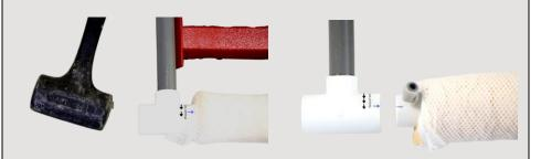
Hammer the sponge white caps into the t-risers until the edge of the white cap reaches the center of the t-riser. Remove the red cap after hammering and shine a flashlight through the riser to make sure your cap has reached the center of the t-riser as shown below.
