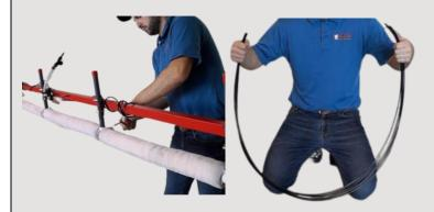
Coil your excess tubing around your boom. Secure with zip ties Simply push the tubing into the quick connectors on both your sponge section, and your manifold (as shown above). Any extra tubing can be coiled up and zip tied down to the boom. Do not over tighten the zip ties and pinch the tubing.
