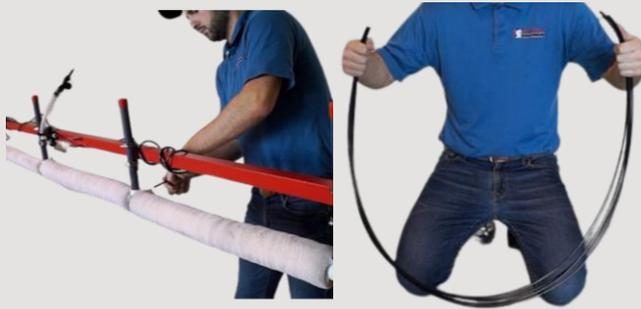
Simply push the tubing into the quick connectors on both your sponge section, and your manifold (as shown above). Any extra tubing can be coiled up and zip tied down to the boom. Do not over tighten the zip ties and pinch the tubing. **Note the manifold in the pictures is a 4-port manifold, you have two 8-port manifolds.**
