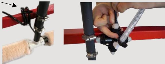
To remove the tubing **hold down the grey ring around push to connect, while pulling out the tubing.**
