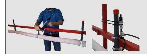
Find the center of your 5 ft. boom. Zip tie it in a secure position. Note pictured position may not be your center. The picture is only meant for visual reference of a secure position
