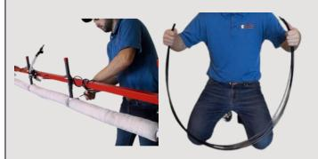
Coil your excess tubing around your boom. Secure with zip ties Simply push the tubing into the quick connectors on both your sponge section, and your manifold (as shown above). Any extra tubing can be coiled up and zip tied down to the boom. Do not over tighten the zip ties and pinch the tubing. The manifold pictured below is a 4-port manifold, your manifold is a 2-port manifold.
