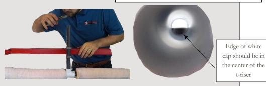
**IMPORTANT:** <u>DO NOT</u> glue your sponge sections into your PVC t-risers. You can pull back your sponges to confirm that the precision drilled holes are pointing in the same direction as shown below.
